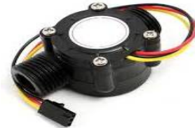
Figure 2. Water Flow Sensor
